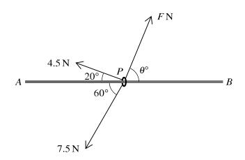
A small ring P is threaded on a fixed smooth horizontal rod AB. Three horizontal forces of magnitudes  $4.5 \,\mathrm{N}, 7.5 \,\mathrm{N}$  and  $F \,\mathrm{N}$  act on P (see diagram).
